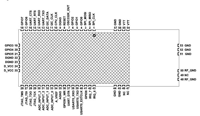
Figure 5-3. Atmel ATZB-A24-U0B Pinout.
