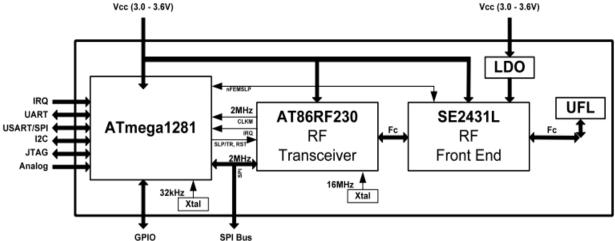
ZigBit Amp modules contain the Atmel ATmega1281V Microcontroller [4] and AT86RF230 RF Transceiver [5]. The module features 128KB flash memory and 8KB RAM.
