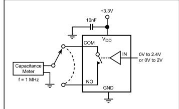
Figure 4. Channel On/Off Capacitance
