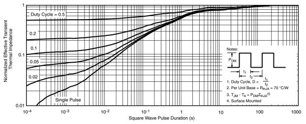
Normalized Thermal Transient Impedance, Junction-to-Ambient
