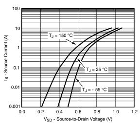
Source-Drain Diode Forward Voltage
