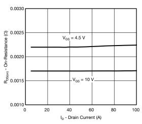
On-Resistance vs. Drain Current
