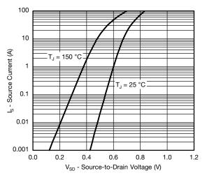
Source-Drain Diode Forward Voltage
