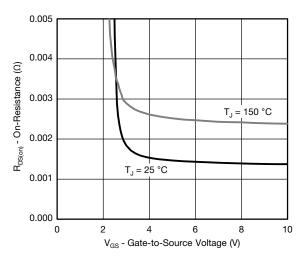
On-Resistance vs. Gate-to-Source Voltage
