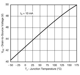
Drain Source Breakdown vs. Junction Temperature
