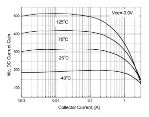
Figure 3. DC Current Gain, Vce=3V
