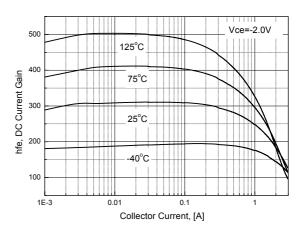
Figure 2. DC Current Gain, Vce=2V
