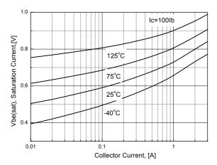
Figure 6. Base-Emitter Saturation Voltage
