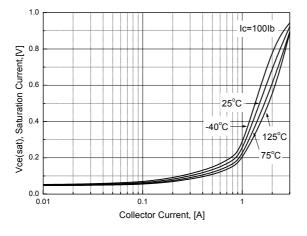
Figure 5. Collector-Emitter Satuation Voltage(2)
