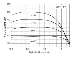
Figure 1. DC Current Gain, Vce=1.5V
