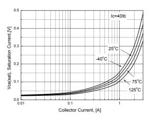
Figure 4. Collector-Emitter Satuation Voltage(1)
