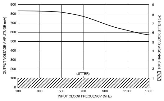
Figure 2. Output Voltage Amplitude (V<sub>OUTpp</sub>)/RMS Jitter vs. Input Clock Frequency at Ambient Temperature
