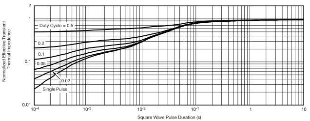
Normalized Thermal Transient Impedance, Junction-to-Foot
