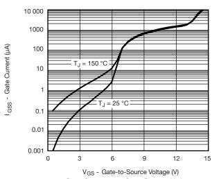
Gate Current vs. Gate-Source Voltage
