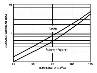
FIGURE 2A. LEAKAGE CURRENT vs TEMPERATURE
