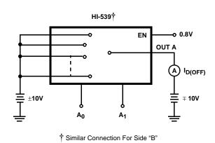
FIGURE 2B. I<sub>D(OFF)</sub> TEST CIRCUIT (NOTE 6)
