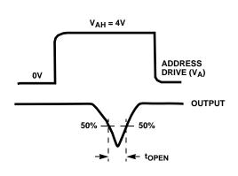
FIGURE 5A. MEASUREMENT POINTS
