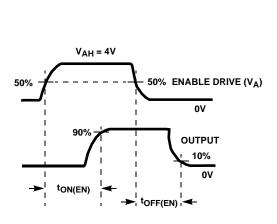
FIGURE 6A. MEASUREMENT POINTS
