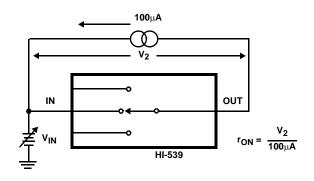
FIGURE 1A. TEST CIRCUIT
