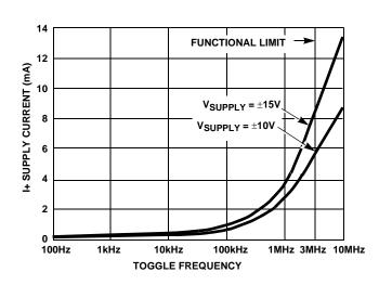
FIGURE 3A. SUPPLY CURRENT vs TOGGLE FREQUENCY
