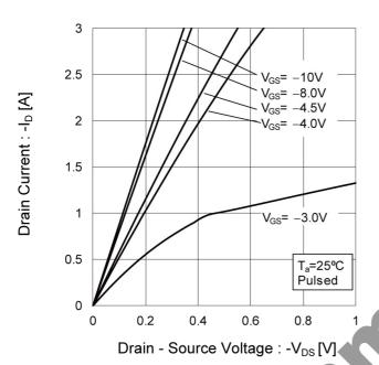
Fig.6 Typical Output Characteristics(II)
