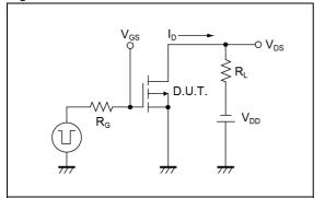
Fig. 2-1 GATE CHARGE MEASUREMENT CIRCUIT
